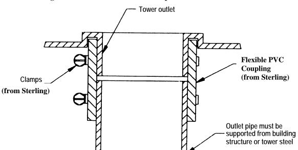
**Figure 5: Flexible PVC Outlet Coupler**
